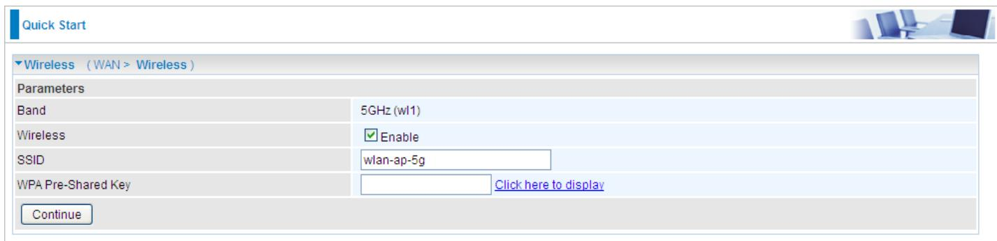
The screenshot shows the 'Wireless' configuration interface for the 5GHz band. The 'Parameters' section includes: Band (5GHz (wl1)), Wireless (Enable checked), SSID (wlan-ap-5g), and WPA Pre-Shared Key (input field and 'Click here to display' link). A 'Continue' button is at the bottom.
