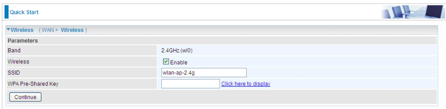
The screenshot shows the 'Wireless' configuration interface for the 2.4GHz band. The 'Parameters' section includes: Band (2.4GHz (wl0)), Wireless (Enable checked), SSID (wlan-ap-2.4g), and WPA Pre-Shared Key (input field and 'Click here to display' link). A 'Continue' button is at the bottom.
